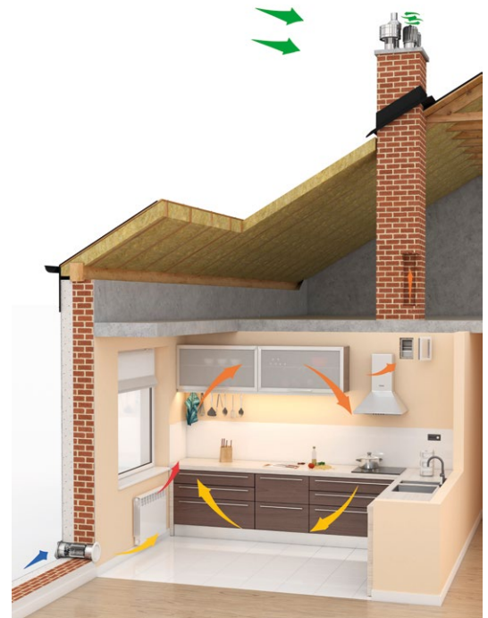
Hybrid ventilation system in single-family housing
